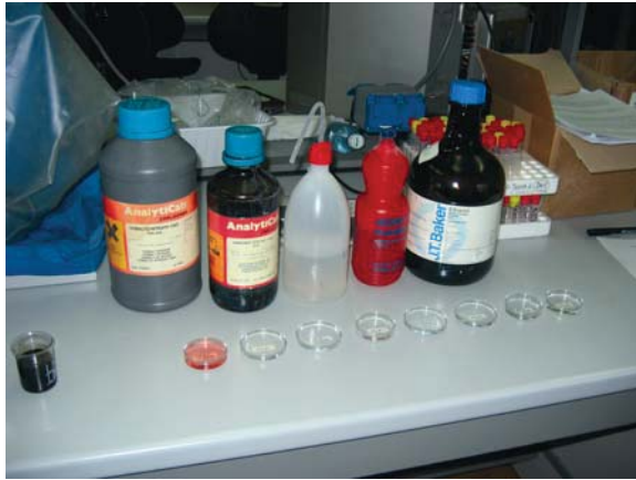
Figure 15. Preparation of cobalt nitrate and ammonium sulphide stain
