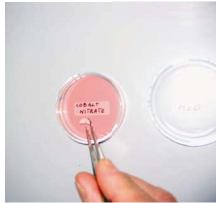
Figure 16. Cleaned vertebra immersed in cobalt nitrate solution
