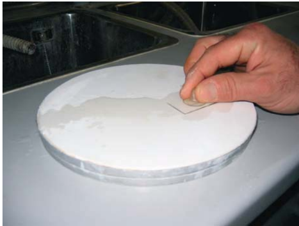
Figure 8. Section polished with finer grit paper to remove scratches
