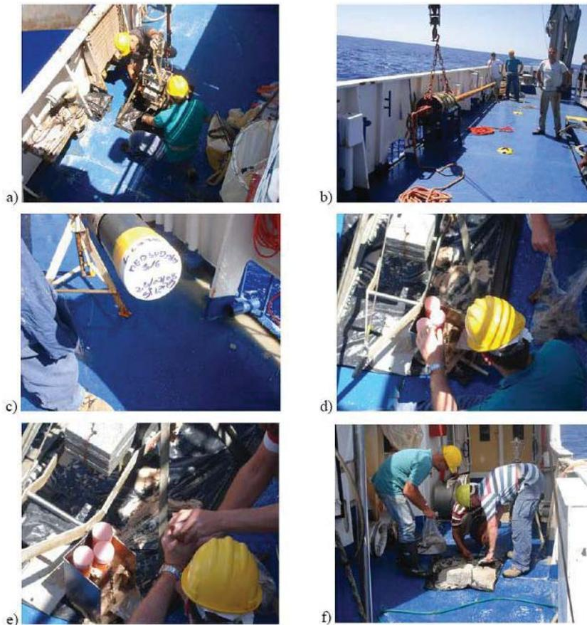
Figure 12.1.1. Sampling with the box corer: PVC tubes and plastic bags.
