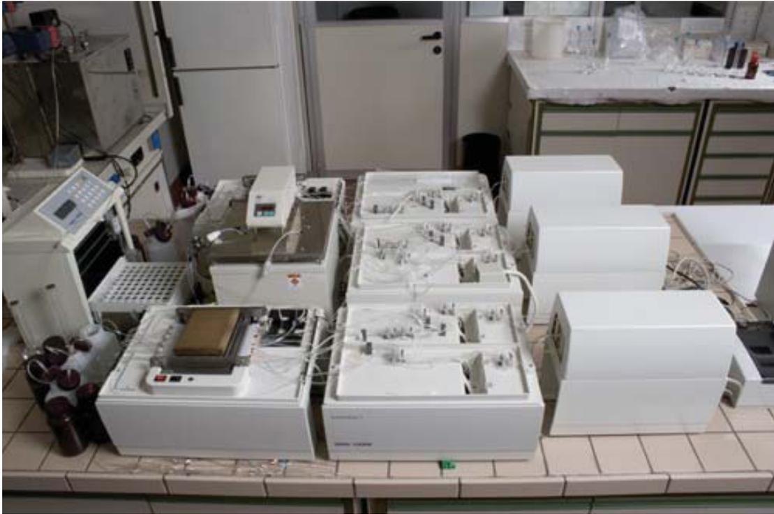
Figure 6.2.1. *AutoAnalyzer III (Continuous Flow) Bran+Luebbe*
