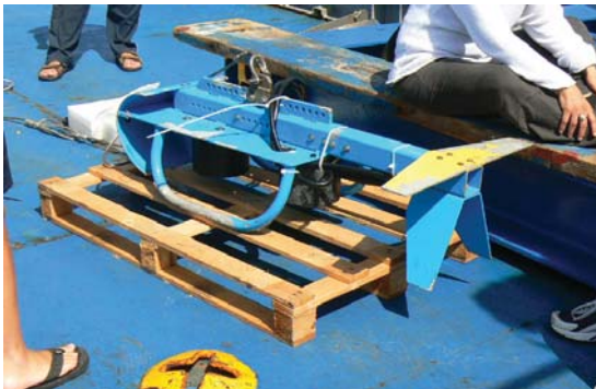
Figure 7. Biosonics DTX Echo-sounder with 2 transducers
