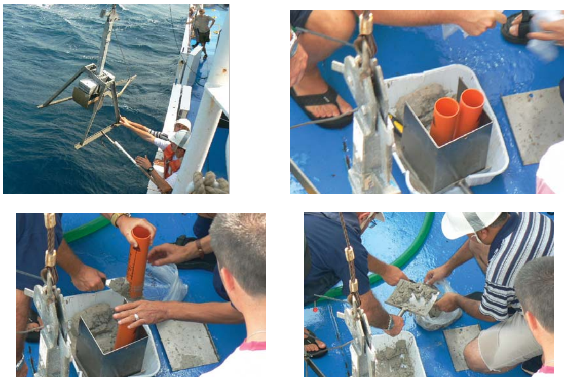
Figure 27. Different steps of the sampling with the box corer: PVC tubes and plastic bags
